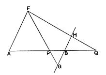
Through A and B draw a pair of parallel lines AF, BH. And through P draw a straight line FPG in any direction meeting AF in F and BH in G. In BH take the point H, so that B is the middle point of GH, and join FH.
